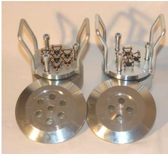
Stressing Heads for tensioning and testing strands
